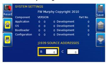
The yellow **Up** and **Down** keys on the left allow you to move the cursor through 'J1939 Source Addresses' fields. While the cursor is highlighting a field, the gray **Up** and **Down** keys scroll through available options. Once all the options have been selected, press **Save**.
