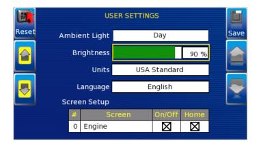
**NOTE**: Brightness level will change with ambient light setting. Two brightness levels are saved; one for day and one for night.
