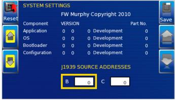
4. With the cursor highlighting the J1939 source addresses, use the left side soft keys to scroll through the ports and the right side soft keys to change the address. Press the
