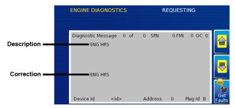
The Engine Diagnostics option displays faults based on engine or auxiliary source.
